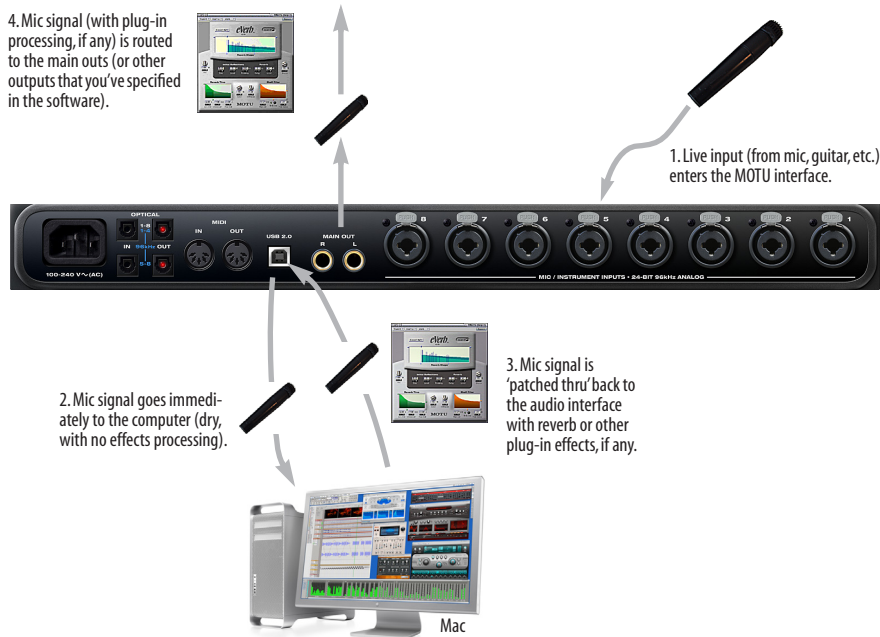
Figure 8-1: There are two ways to monitor live audio inputs with an 8pre USB: 1) through the computer or 2) via CueMix™ DSP hardware monitoring. This diagram shows method 1 (through the computer). When using this method, use your host software’s buffer setting to reduce the slight delay you hear when monitoring the live input, but don’t lower it too much, or your computer might get sluggish.
