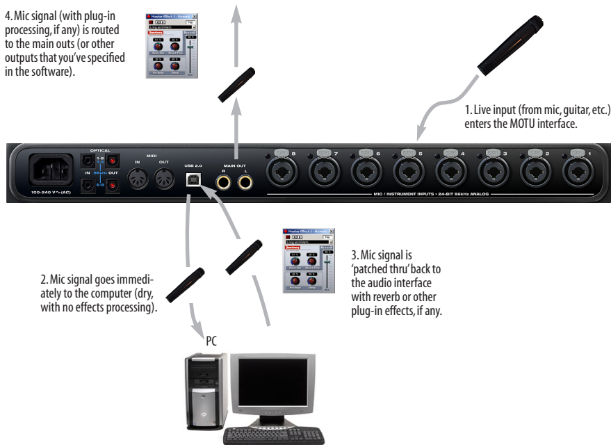
Figure 8-1: There are two ways to monitor live audio inputs with an 8pre USB: 1) through the computer or 2) via CueMix™ DSP hardware monitoring. This diagram shows method 1 (through the computer). When using this method, use MOTU Audio Console's buffer setting (Figure 8-3 on page 43) to reduce the slight delay you hear when monitoring the live input, but don't lower it too much, or your computer might get sluggish.
