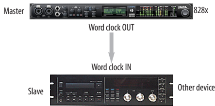
Figure 4-17: Slaving another digital audio device to the 828x via word clock. For the 828x clock source, choose any source besides word clock, as it is not advisable to chain word clock.
