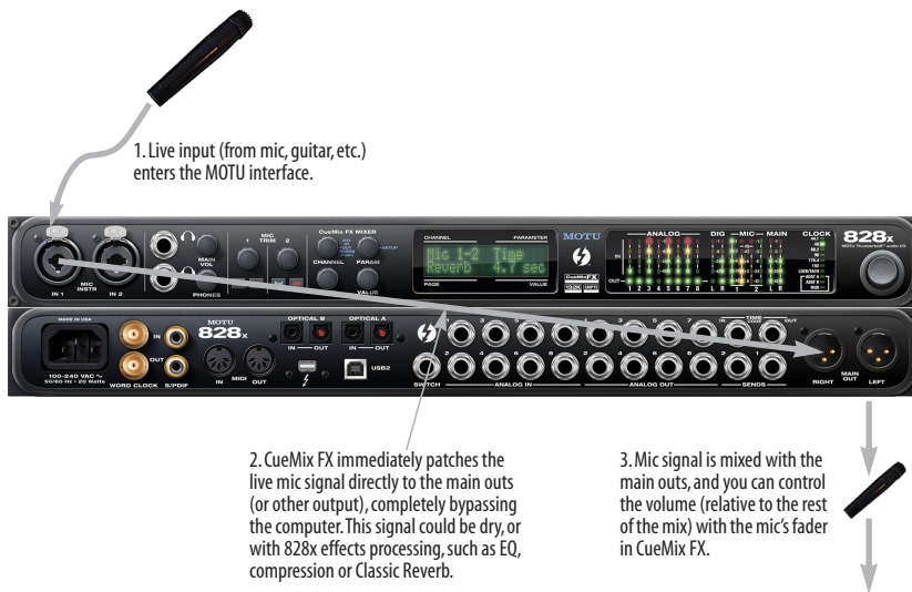
Figure 8-2: This diagram shows the signal flow when using CueMix FX no-latency monitoring. Notice that this method does not process the live input with plug-ins in your audio software. Instead, you can apply 828x effects, such as the reverb, EQ and/or compression.
