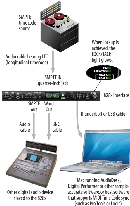
Figure 4-15: Connections for synchronizing the 828x directly to SMPTE timecode.
