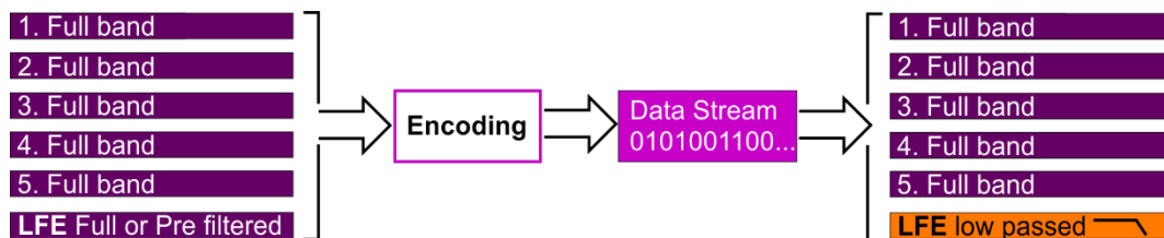
Figure 1 - Audio bandwidths of encoded 5.1 channel materials
